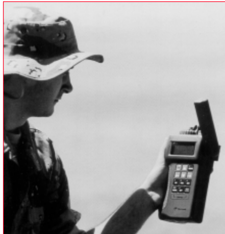
A military handheld GPS receiver (courtesy Rockwell)
